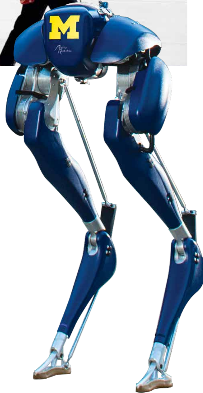
U-M's bipedal robot Cassie Blue, built by Agility Robotics, sports five motors in each leg, four hours of battery life, and weighs only 73 pounds. Cassie utilizes code from its predecessor, MARLO.
