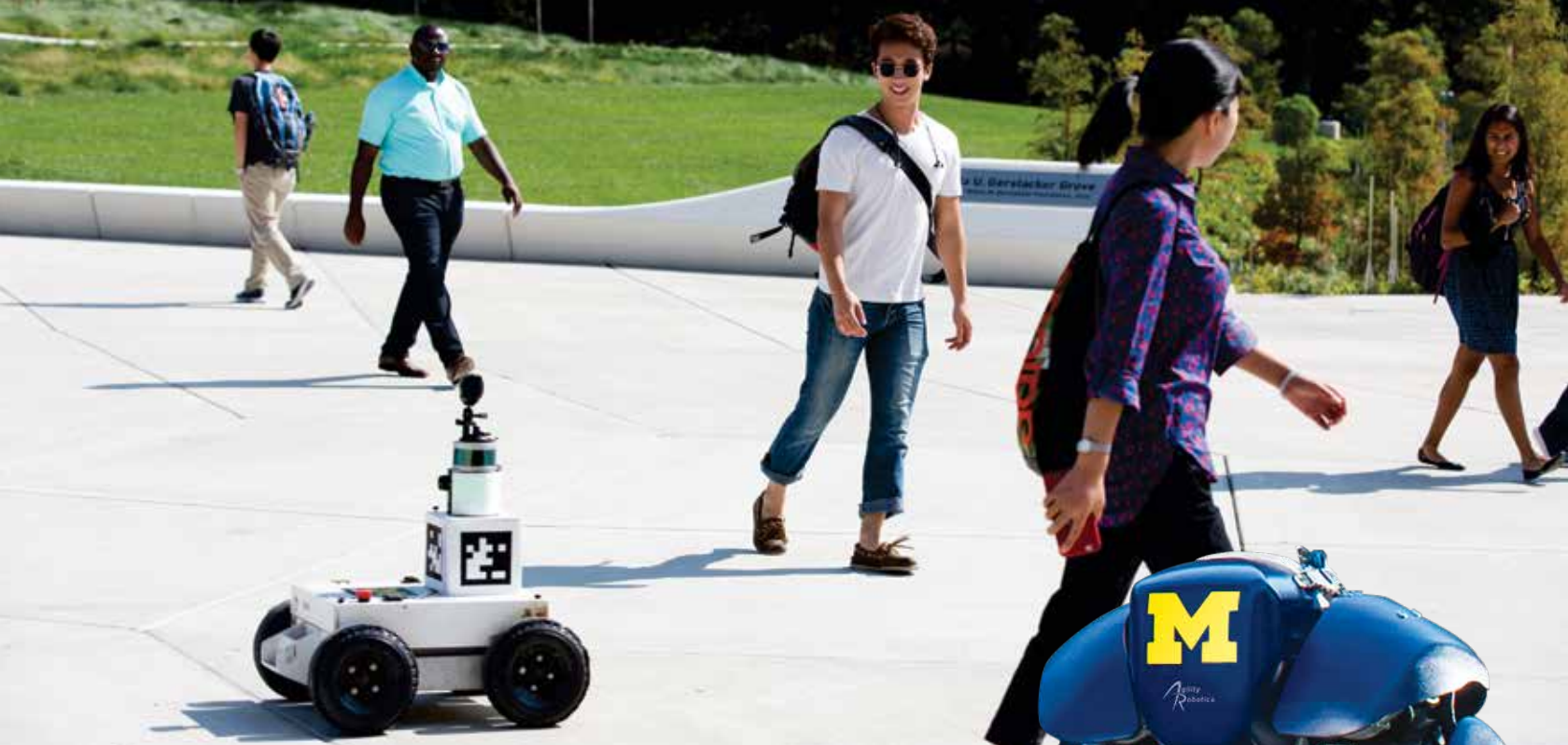
Team Michigan's award-winning MAGIC (Multi Autonomous Ground-robotic International Challenge) robot explores the Eda U. Gerstacker Grove on North Campus. New technology enables the robot to autonomously analyze the environment and determine its optimal path.
